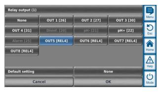
The figure shows an example of a menu for the assignment of a relay switch output.
