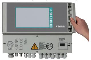
Remove the cover plate and unhook the hinge on the bottom.
