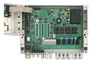
Dismantle the cable (or cables) on the required length inside the casing and insert it (them) into the casing through one or more cable glands.
